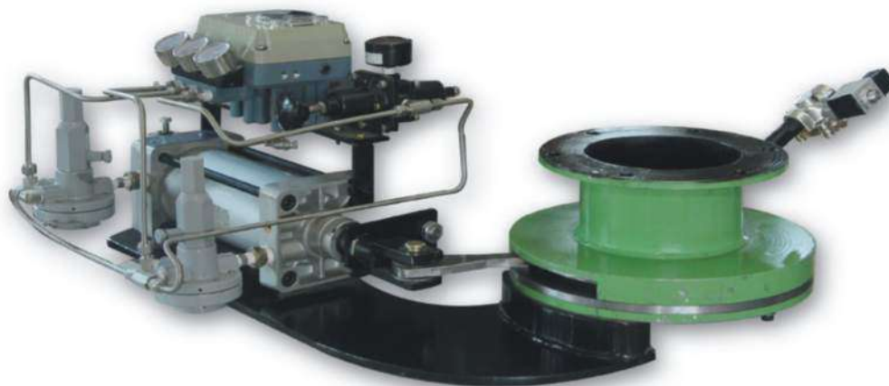
YUTECH Concentric Split Diaphragm (CSD) Control Valve Also called Iris Type Control Valve with Pneumatic Linear Actuation using Electro-Pneumatic Positioner
