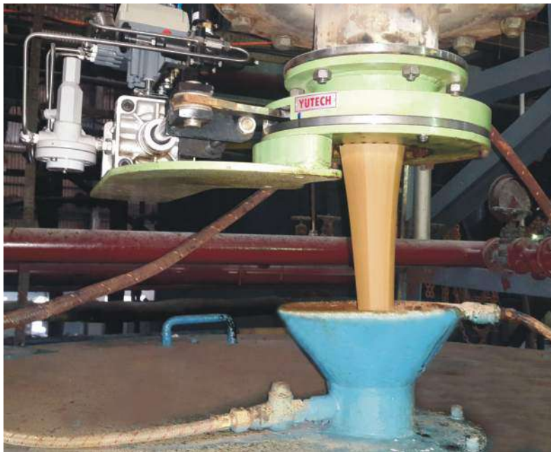
YUTECH CSD Pneumatic Control Valve Automatically Feeds Continuous Centrifugal Machine
