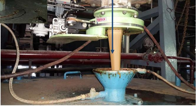
CSD OR IRIS VALVE BASED CONTINUOUS CENTRIFUGAL MACHINE FEED AUTOMATION SYSTEM
