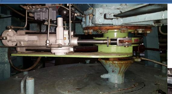
Controlled Quantity of Massecuite drops from the Concentric Opening (Split opening from the Centre of the Valve) Hence No Spilling, No Splattering, No Unbalance, No Overflow, No Underfeeding
