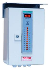
Field Mounted Ethernet Scanner is a system designed for convenience. It eliminates, Termination Blocks, Junction Boxes, and Wiring required for each of these devices. All Sensor / Transmitter Signal Wires are Terminated in this Scanner, and the Ethernet Cable can be taken to PLC / DCS / Computer saving a huge quantity of Wires and Labour. It can be terminated in the Ethernet side of your Fibre Optic Network for long-distance communications.
